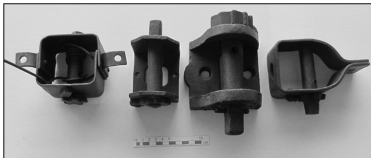
Figura 25: tensor Magerand, llaves “californianas” y tensor Grip o Pilter.
