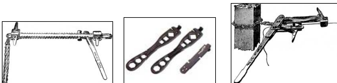
Figura 25: tensor Magerand, llaves “californianas” y tensor Grip o Pilter.
