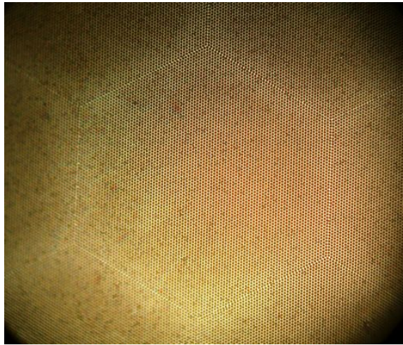
Figure 26: Picture of an MCP with the hexagonal structure due to fabrication fashion. The structure causes a modulation in the individual pixel gain of 24 pixels for the FM.
