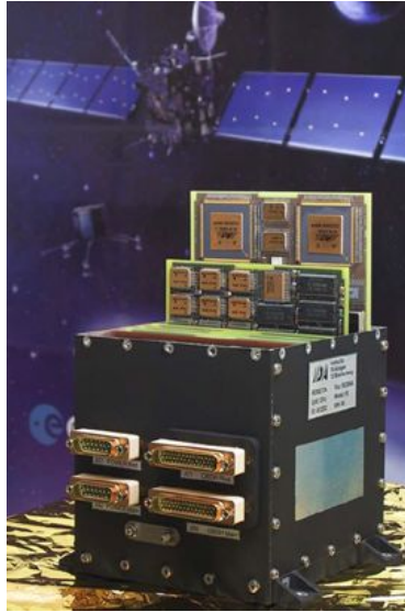
Figure 13: Digital Processing Unit (DPU). Image credit: Balsiger et al. (2007)
