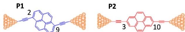
Fig. 1 Two molecules P1 and P2 with common pyrene hearts, but different connectivities to gold electrodes. (See figure 2 for a more detailed numbering convention used in this study. This does not correspond to the usual chemical numbering convention, but it is convenient analytically and allows us to assign labels to all atoms.)
