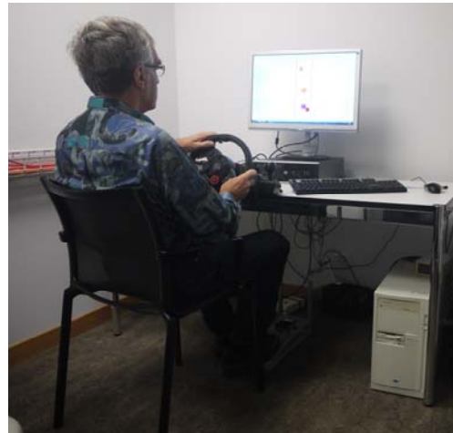
Fig. 1 Setup of the BCST with screen, steering-wheel, and foot-pedal.
