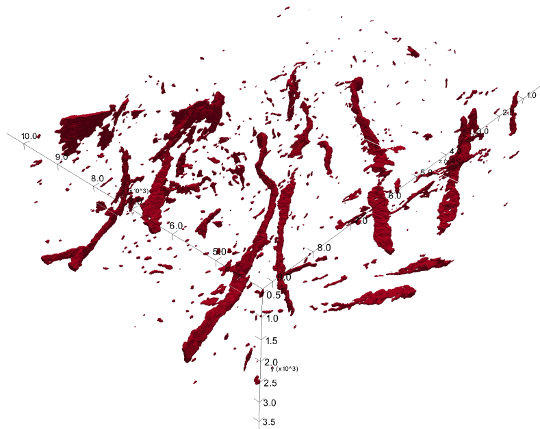
Figure 7.9: Segmented porosity from a FIB/SEM tomography of a volume of 3.5 \mu\text{m} \times 5 \mu\text{m} \times 10 \mu\text{m} from a bovine cortical bone sample (by courtesy of Joan Rovira, PhD).
