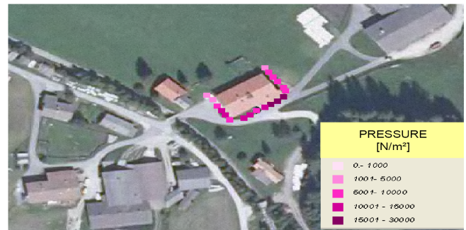
Figure 14. Representation of maximum pressure values in \text{N m}^{-2} on the building envelope.
