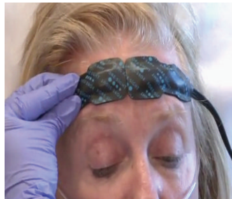
FIGURE 4: The Fore-sight monitor for cerebral blood flow in stroke treatment. Courtesy of Casmed, Brandford, CT, USA.
