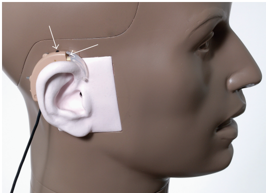
FIGURE 2: Behind-the-ear housing containing the two-omnidirectional microphones (arrows) mounted on KEMAR manikin.
