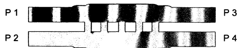
Fig. 1. Layout of a 90° branchline coupler. The colors represent the simulated electrical field when a signal is injected at port 1.
