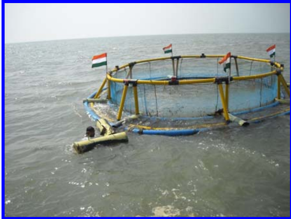
Fig.1: Circular 6 m diameter HDPE cage launched at Kalamb, Thane District.
