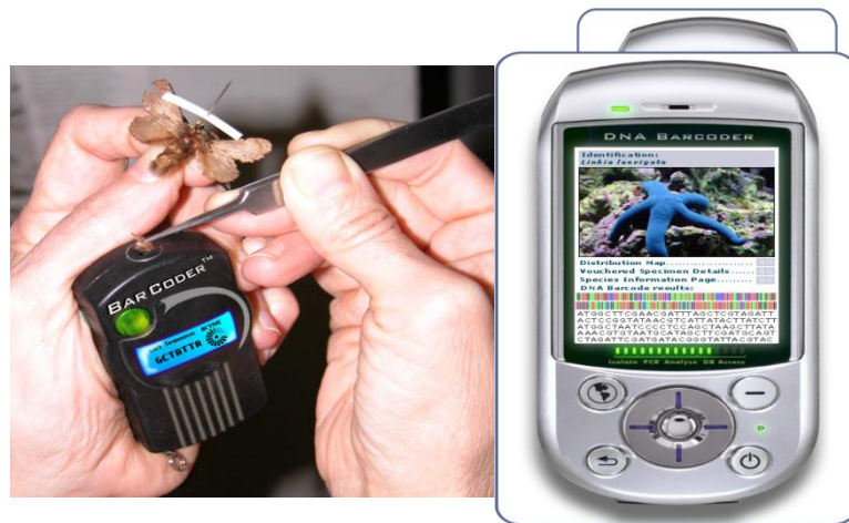
Fig 12. 2. Two prototypes of hand-held DNA Barcoder (by 2015?). (Source: http://www.barcodinglife.org/views/login.php )
