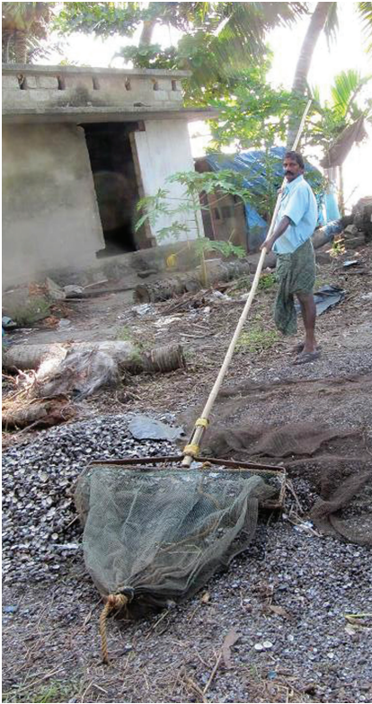
Figure 10a.—Fisherman holding a hand rake used from a canoe to harvest black clams. Its teeth are 7.5 cm (3 in) long; there are 70 teeth; its nylon mesh netting has holes 1.5 cm (0.5 in) wide; the pole is 5 m (16 ft) long; weight hand rake is 6.8–9 kg (15–20 lbs). A complete new rake costs about Rs.1, 000 (US$22).
