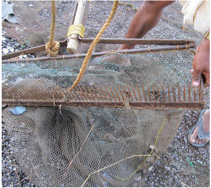
Figure 10b.—Close-up of hand rake for harvesting black clams showing some of its teeth and net to hold the clams.
