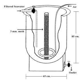
Fig. 1 Diagram illustrating the dimensions and arrangement of inflow and out flow of water and aeration for rearing H. kuda young ones
