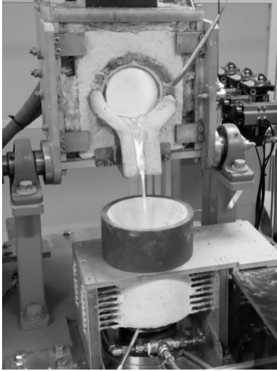
Figure 7. Crucible set-up and pouring of molten liquid of metallic alloy
