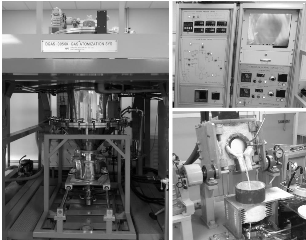
Figure 5. Gas atomization system and peripherals
