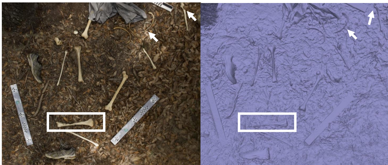
Figure 31. Zoomed in screenshot of the texture (left) and geometry (right) of the lower leg portion of Model 1. The arrows show poor ground surface-subject interface in the areas of the left ulna (top right) and the unserialised ribs (left). The white box is showing the misrendered geometry of the left tibia.
