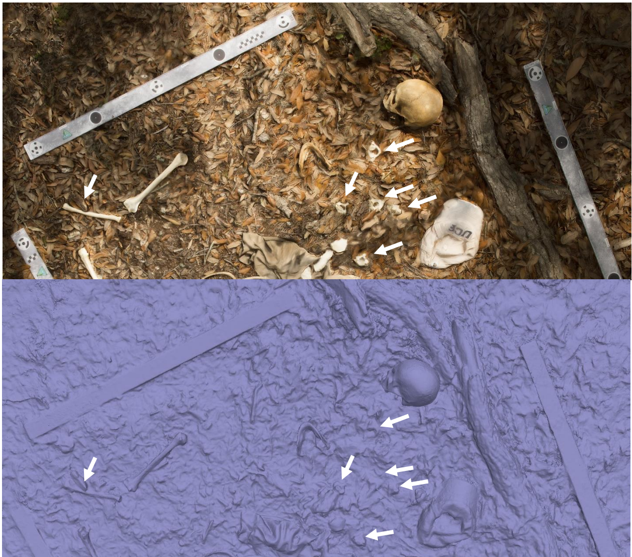
Figure 37. Screenshots of the textured (top) and geometry (bottom) of the head section of Model 3. White arrows are pointing out the ground surface-subject interfacing error in the right humerus (left) and the unserialized cervical vertebrae (right).
