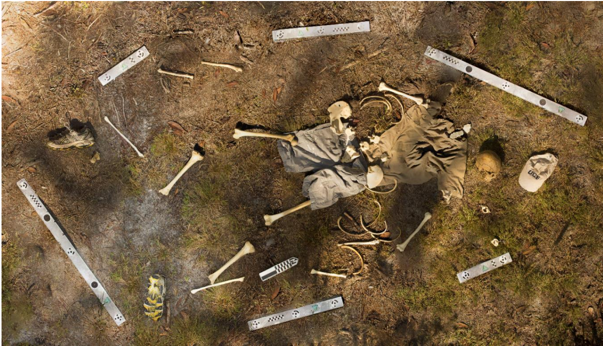
Figure 50. Second orthophoto generated for Model 4 by manually inspecting and removing photographs from the program. This orthophoto shows improvement in the shadows over the scene as well as the removal of the scale distortion and the feet of the researchers.
