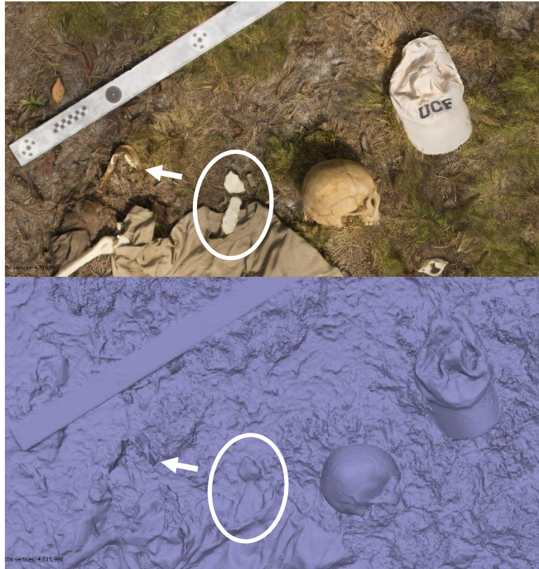
Figure 45. Zoomed in screenshots of Model 4 showing both the textured (top) and mesh (bottom) models. The oval shows the subject-subject interface issue connecting the manubrium and the body of the sternum, and the arrow shows the misrendered geometry on the right ascending ramus of the mandible.
