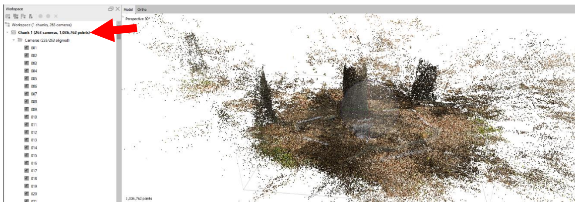
Figure 14. The resulting SPC in the viewing window of Agisoft Metashape Professional. In case any mistakes are made in the optimization, duplicate the chunk by right clicking on the chunk title (red arrow) and choose “Duplicate Chunk”.
