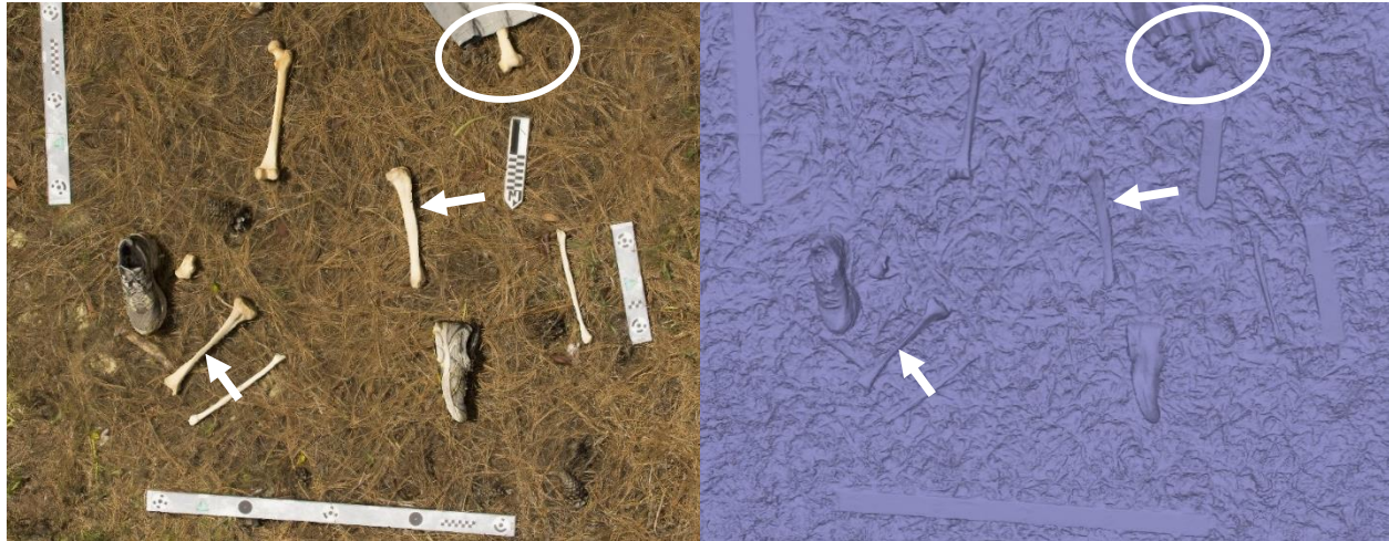
Figure 55. Slightly zoomed in overhead screenshot of the lower legs of Model 5 showing both the textured (left) and mesh (right) models. The arrows show areas of slight misrendered geometry on the left and right tibiae and the oval indicates an area of subject-subject interfacing error between the left femur and pant leg.
