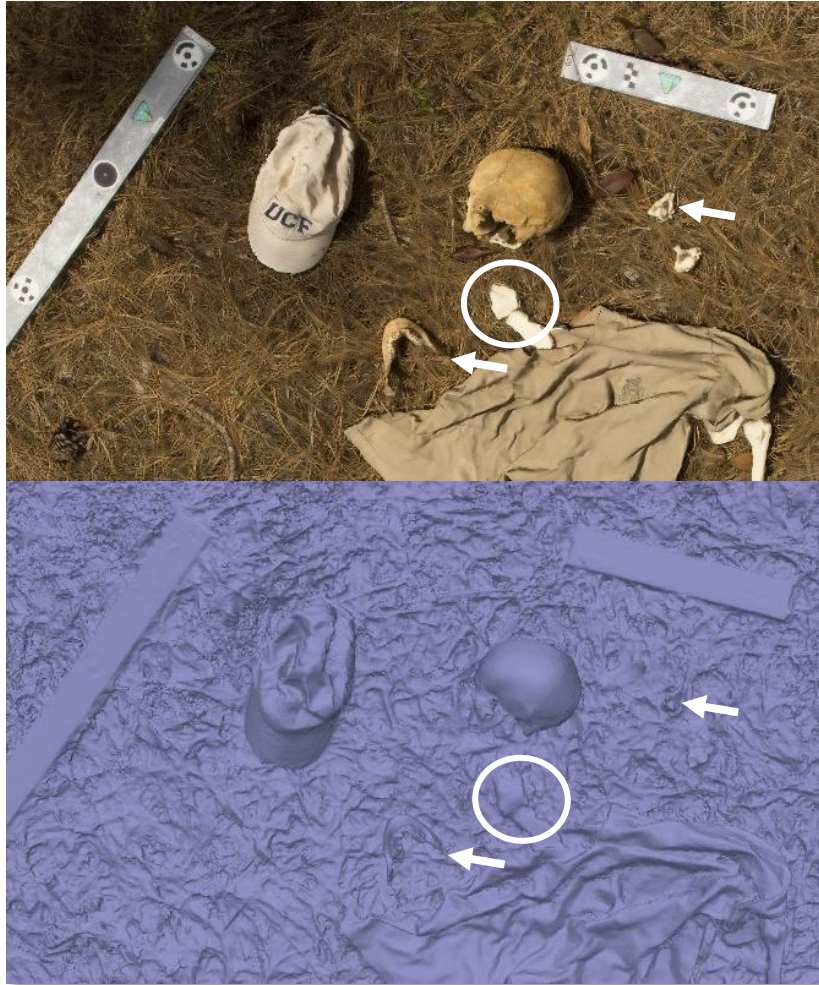
Figure 52. Zoomed in screenshots of Model 5 showing both the textured (top) and mesh (bottom) models. The left arrow shows an area of misrendered geometry on the right ascending ramus of the mandible. The oval shows a subject-subject interfacing error between the manubrium and sternal body, and the right arrow shows ground surface-subject interface error between the axis and the ground surface.
