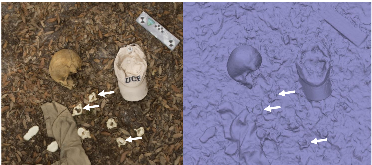
Figure 58. Zoomed in screenshots of Model 6 showing both the textured (left) and mesh (right) models. The arrows show the ground surface-subject interfacing errors between the cervical vertebrae and the ground surface.
