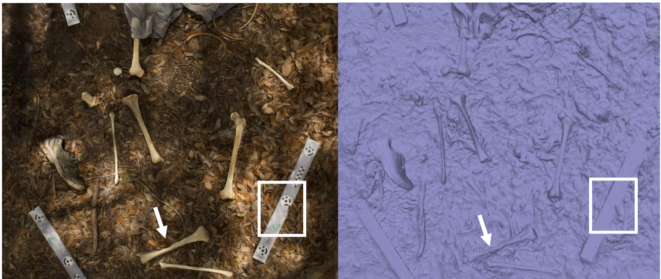
Figure 39. Screenshots of the texture (left) and geometry (right) layers of the lower leg portion of Model 3. White arrow showing the misrendered geometry on the left tibia, and the white box showing the ground surface-subject interfacing error on the scale bar due to leaf litter covering.
