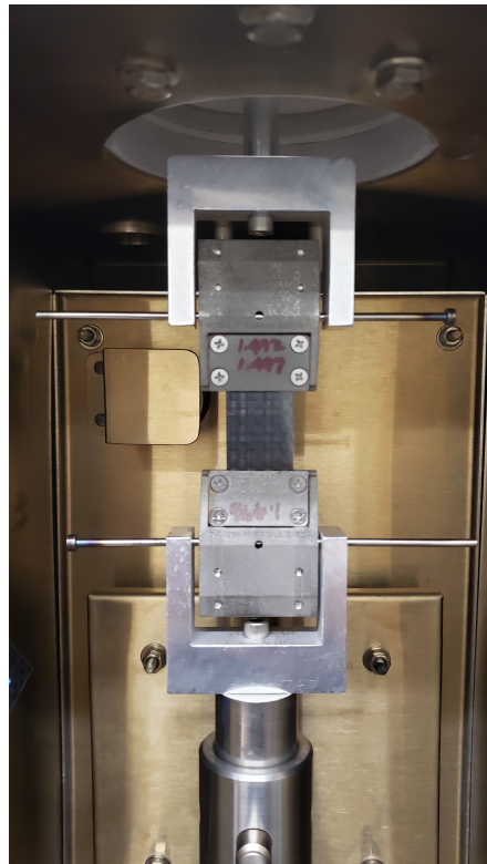
Figure 3.3: Column Bending Test setup
