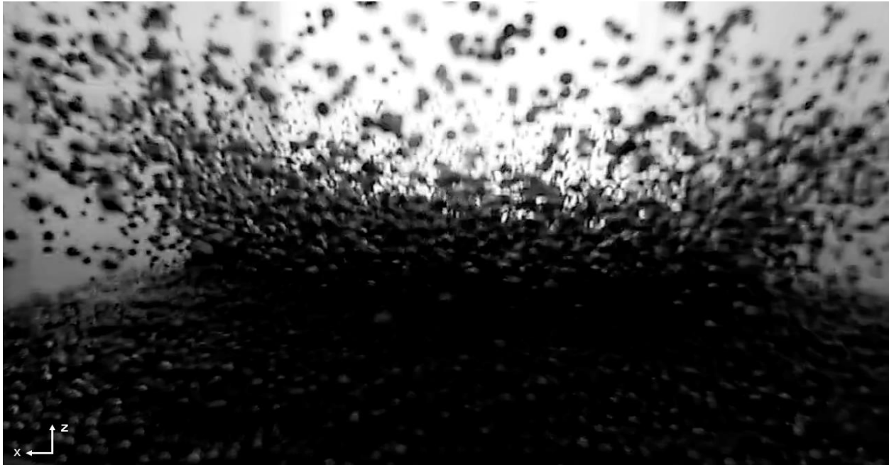
Figure 31: Side view, 292 ms into a 250 ms pulse experiment in \mu\text{g} . At this nozzle height we see a shallow ejecta angle, possibly exacerbated by the shallow simulant depth.
