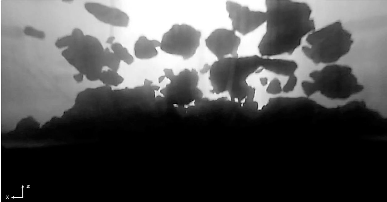
Figure 47: A side view of CI Orgueil simulant lofted in a 50 ms pulse \mu\text{g} experiment, seen here 375 ms after jetting was triggered. Compare the significant increase in ejecta to lower jetting durations.
