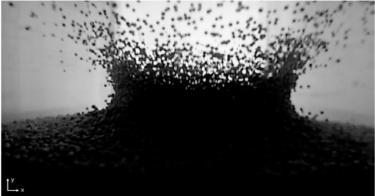
Figure 34: Side view, 200 ms into a 100 ms pulse experiment into steel beads in \mu\text{g} . The ejecta splash smoothly transitions into the undisturbed surface.
