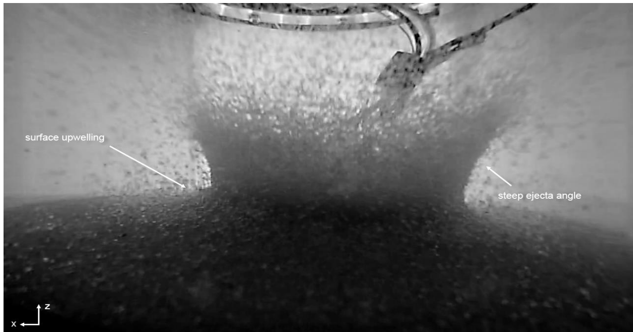
Figure 43: Well-defined ejecta from a 50 ms pulse into glass beads from 15 cm, here at 125 ms into the experiment in \mu g. Off-center lofting is also visible outside the primary ejecta wall.
