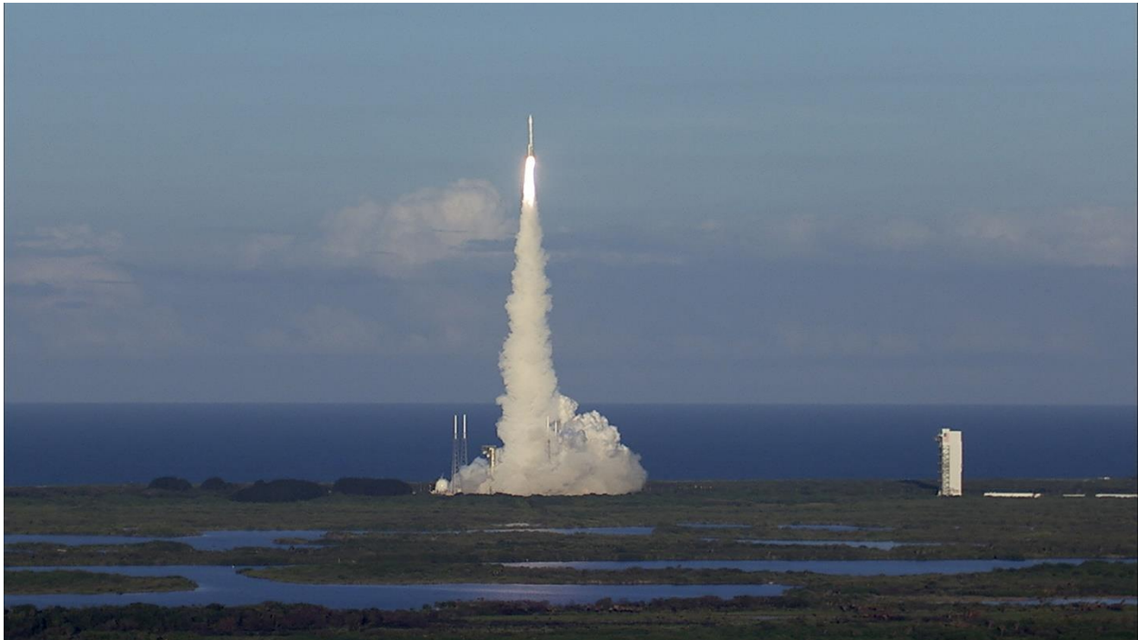
Figure 1: The exhaust plume trails out beneath this Atlas V rocket as it launches from the Florida coast. The edges of the plume are rough, indicating turbulent flow due to Earth's relatively thick atmosphere.
