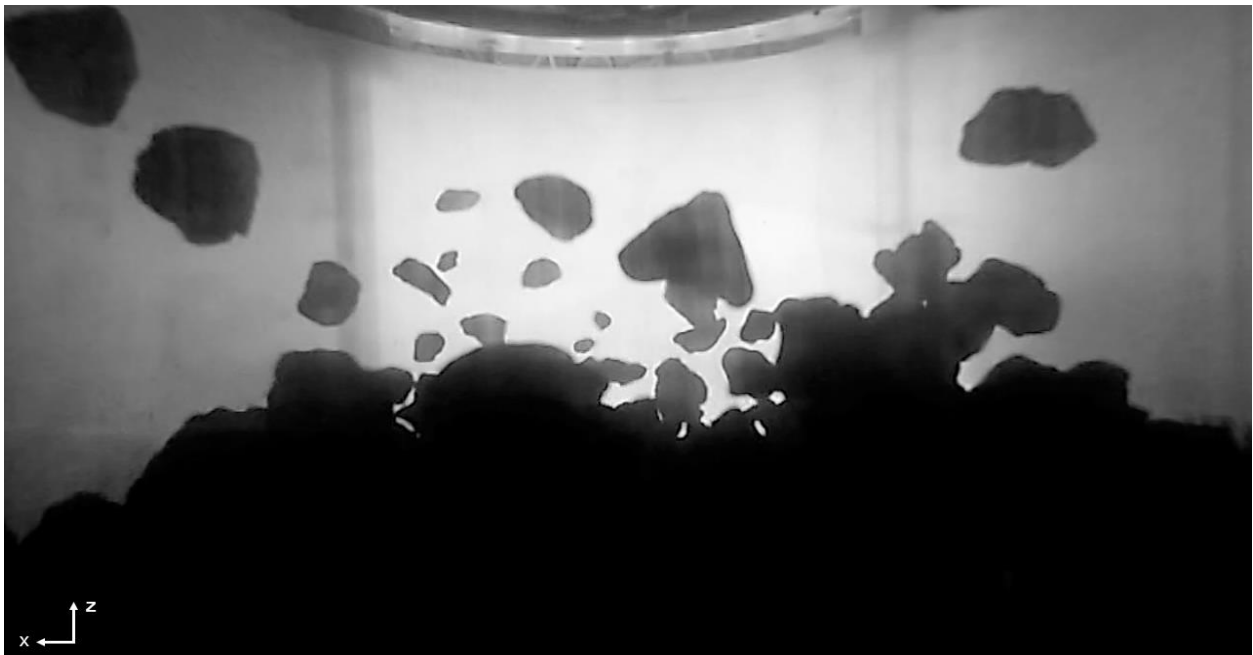
Figure 50: Side view of a 50 ms pulse CI Orgueil \mu\text{g} experiment, seen 375 ms after jetting start. Compare this to Figure 47, which shows the same experiment at 25 cm nozzle height.
