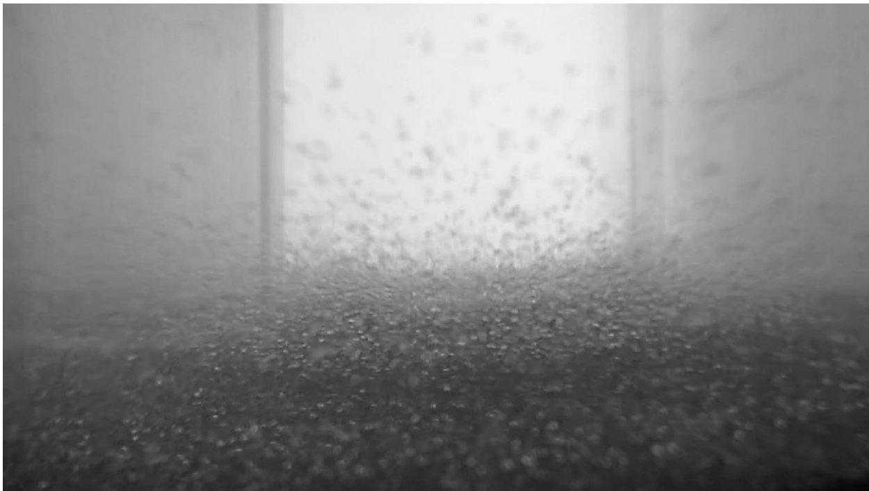
Figure 42: A side view frame of a 50 ms pulse into glass beads in \mu\text{g} , seen here at 83 ms into the experiment. Shallow ejecta splays outward and obscures much of the view.
