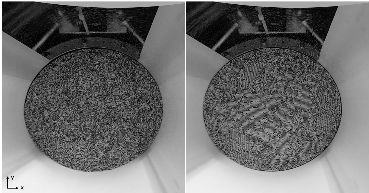
Figure 28: Surface prior to plume impingement. Left, experiment 56, shows a typical initial surface condition. On the right, experiment 55, with a regular packing arrangement visible in the center region.
