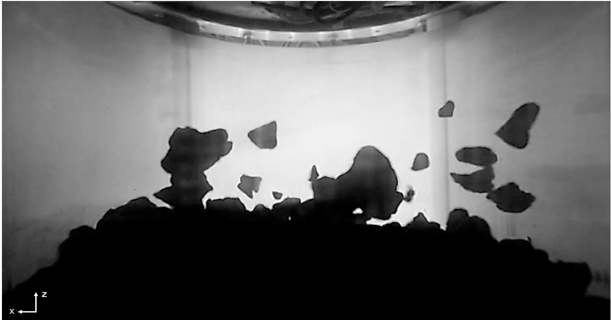
Figure 49: Side view of a 25 ms pulse CI Orgueil \mu\text{g} experiment, seen 375 ms after jetting start. Compare this to Figure 46, which shows the same experiment at 25 cm nozzle height.
