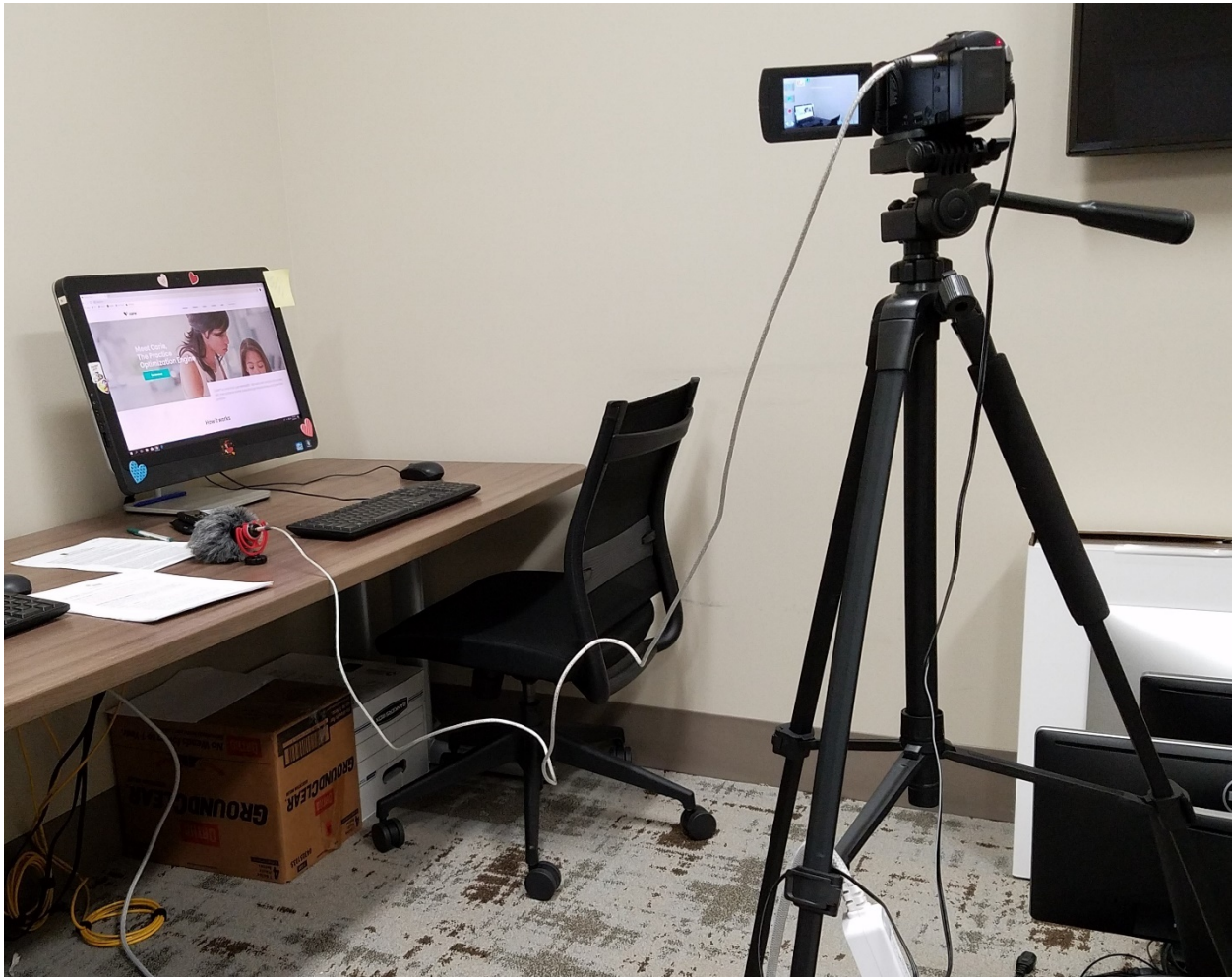
Figure 7: Think Aloud Usability Test Video / Audio Recording Set-up
