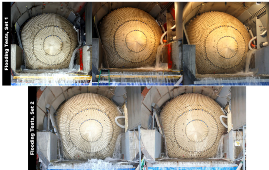
Fig. 13 Phase 2b-ET, full-scale testing, three-layer Vectran plug: Front view of flooding tests carried out for Phase 2b (top row) and Phase 2b-ET (bottom row) [69, 88]
