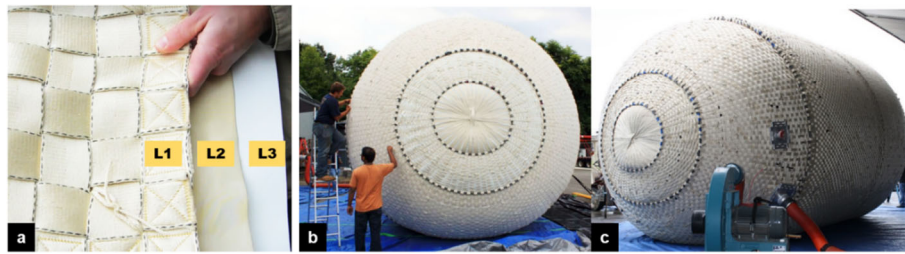
Fig. 6 Phase 2b. a Three-layer membrane configuration comprised of Vectran woven webbing (L1), protective Vectran fabric layer (L2), and inner bladder layer of urethane-coated polyester (L3). Unconfined inflation of (b) full-scale three-layer surrogate plug; (c) full-scale three-layer Vectran plug [44, 87, 88]
