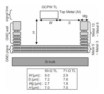
Figure 2. The cross-view of the GCPW-TLs.
