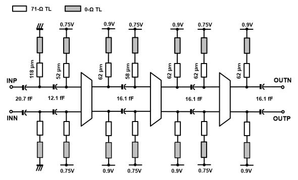
Figure 4. The proposed D-band PA.
