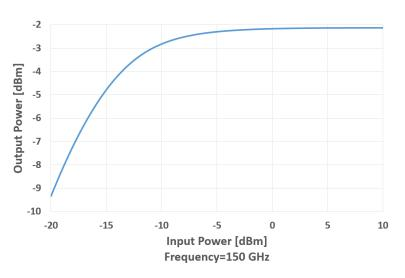
Figure 11. The simulated output power versus input power of the 300 GHz transmitter front-end.
