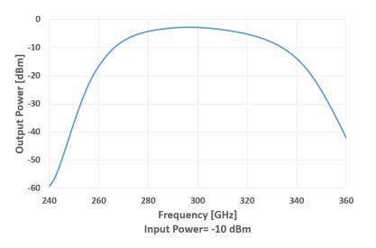
Figure 12. The simulated output power versus output frequency of the 300 GHz transmitter front-end.
