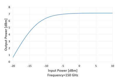
Figure 8. The simulated output power versus input power of the two-way D-band PA.
