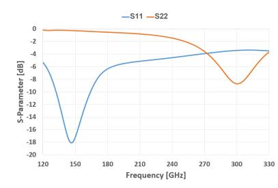
Figure 10. The simulated S-parameter of the 300 GHz transmitter front-end.
