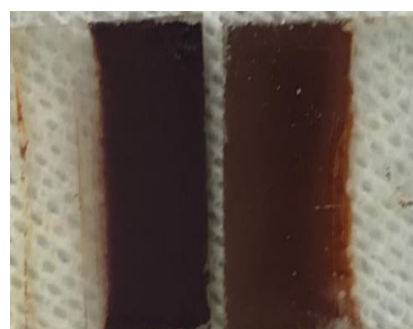
Figure 6. The photo images of the dyed photoanodes with the ozone treatment (left) and without the ozone treatment (right)
