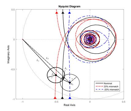
Figure 10. Nyquist plot for  $\pm 20\%$  mismatches in both delay and model parameters  $\omega = 0.6 \ rad/s$ .
