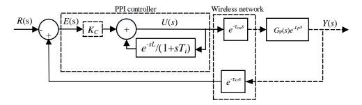
Figure 1. PPI controller in wireless network set-up
