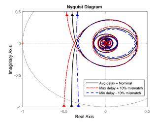
Figure 8. Nyquist plot for mean, maximum and minimum network delays.
