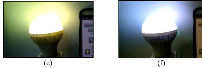
Figure 14. Functional evaluation for ambient lamp driver: (a) red, (b) green, (c) blue, (d) magenta, (e) yellow, (f) white
