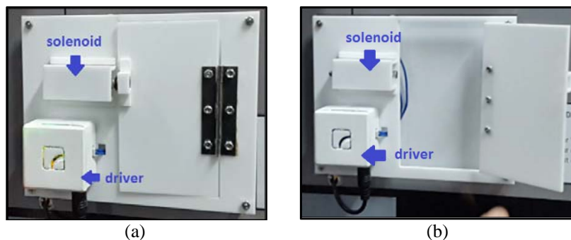
Figure 10. Functional evaluation on door lock driver: (a) locked, (b) opened
