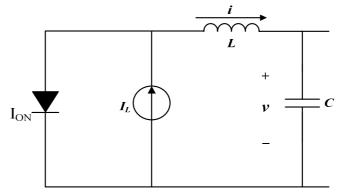
Figure 4. PV equivalent circuit [22]
