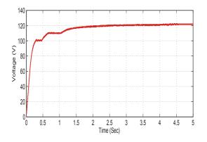
Figure 11. PV cell performance with constant load under constant radiation and temperature (y-axis PV array voltage (V) and x-axis time)
