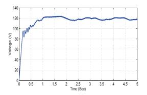
Figure 9. PV cell performance with PHEVs load under constant radiation and temperature (y-axis PV array voltage (V) and x-axis time)
