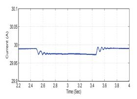
Figure 14. PV cell performance with PHEVs load under variable radiation and temperature (y-axis PV array current (A) and x-axis time)
