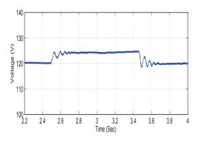
Figure 13. PV cell performance with PHEVs load under variable radiation and temperature (y-axis PV array voltage (V) and x-axis time)
