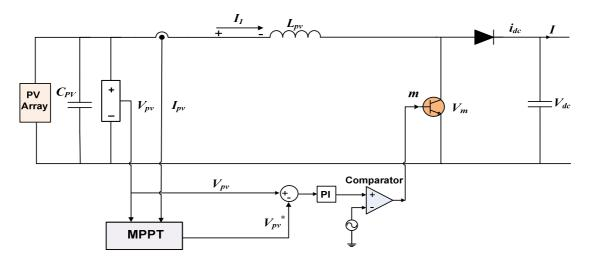
Figure 6. PV converter controller System
