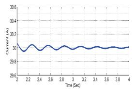
Figure 10. PV cell performance with PHEVs load under constant radiation and temperature (y-axis PV array current (A) and x-axis time)
