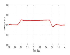
Figure 15. PV cell performance with constant load under variable radiation and temperature(y-axis PV array voltage (V) and x-axis time)
