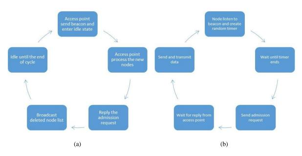
Figure 2. (a) Process flow of access point, (b) Process flow of node
