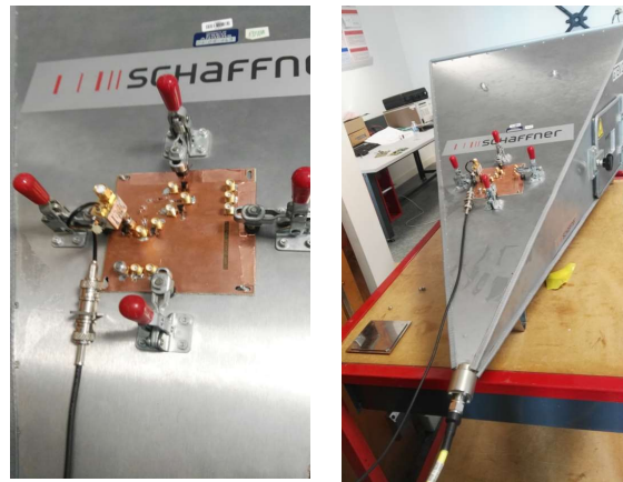
Figure 4. Circuit under test in the GTEM
