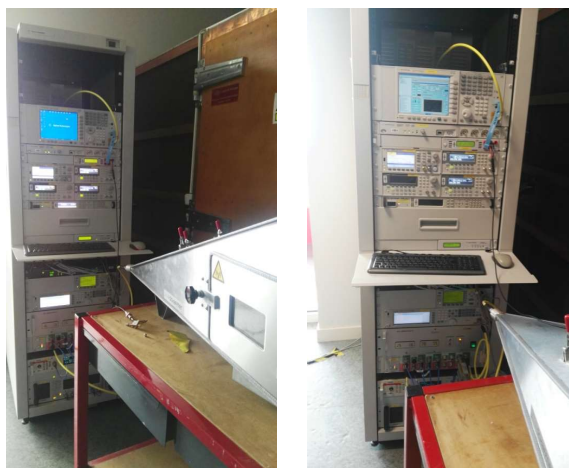
Figure 5. RF generator for immunity measurements of ESEO-EMC Laboratory
