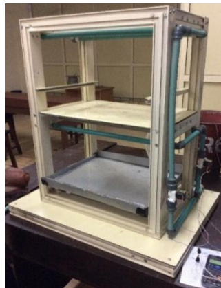
Figure 6. The constructed aluminium framework with piping
