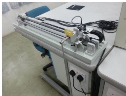
Figure 1. GLIP2001 single inverted pendulum apparatus
