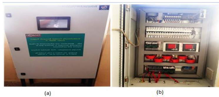
Figure 5. Fabricated hardware model of RTCM device (a) Front interface and (b) Load generators
