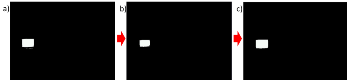
Figure 4. Application of morphological filters. a) Binarized original image. b) Application of the erosion filter. c) Application of the dilation filter.
