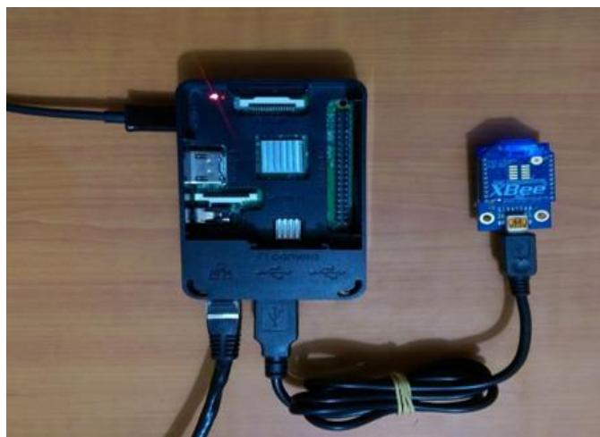
Figure 5. Hardware implementation of the main station node
