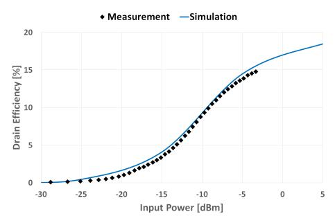
Figure 8. The measured and simulated drain efficiency of the 60 GHz PA.
