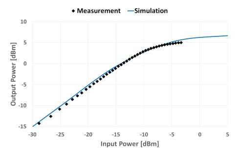
Figure 7. The measured and simulated output power versus the input power of the 60 GHz PA.
