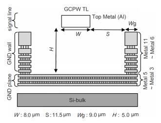
Figure 3. The cross-view of the 50  $\Omega$  GCPW-TL.
