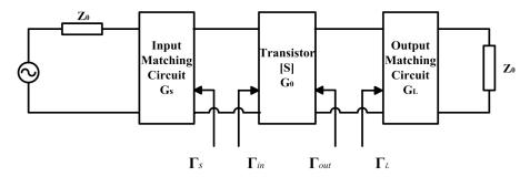
Figure 1. Block diagram of a PA.
