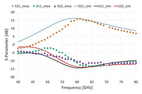
Figure 6. The measured and simulated S-parameter of the 60 GHz PA.
