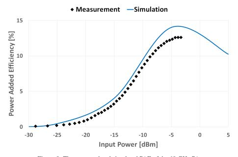
Figure 9. The measured and simulated PAE of the 60 GHz PA.
