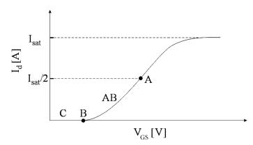
Figure 2. Operating points of different current-mode PAs classes.
