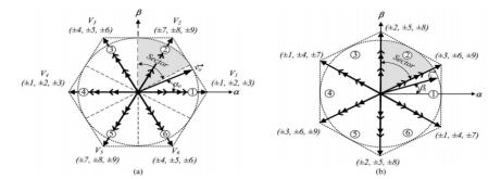
Figure 2. MC vectors. (a) Output voltage vectors. (b) Input current vectors.
