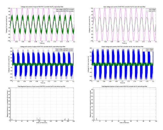
Figure 4. Waveform of voltage and current of MATRIX converter fed RL load
