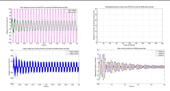
Figure 5. Waveform of voltage and current of MATRIX converter fed PMSM without input filter
