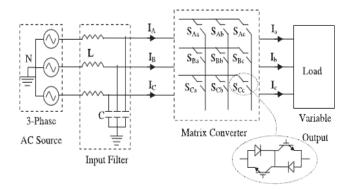
Figure 1. MATRIX converter schematic
