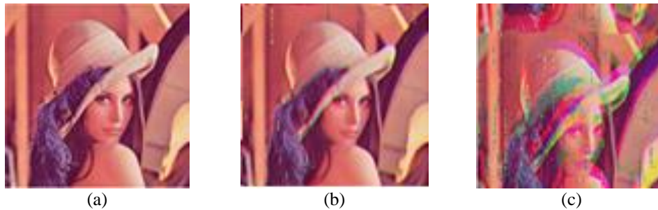
Figure 8. The received Lenna image with different SNR, (a) SNR=10 dB, FFT size=256, PSNR=71.5, (b) SNR=8 dB, FFT size=256, PSNR=20.7147, (c) SNR=6 dB, FFT size=256, PSNR=13.5189
