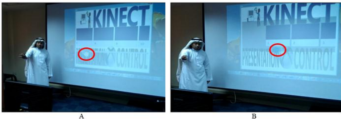
Figure 4. (a) Hand cursor that use for selection, (b) Selecting a thumbnail is indicated with cursor changes colours
