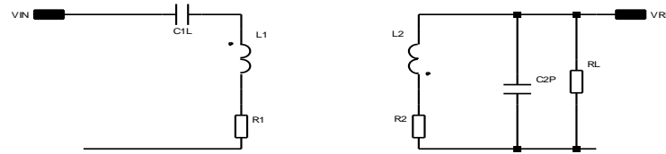
Figure 2. Inductive link topology
