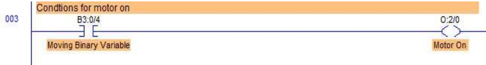
Figure 8. Ladder logic for rung 3
