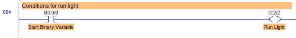
Figure 9. Ladder logic for rung 4
