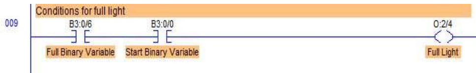
Figure 14. Ladder logic for rung 9
