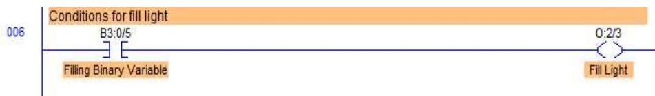
Figure 11. Ladder logic for rung 6
