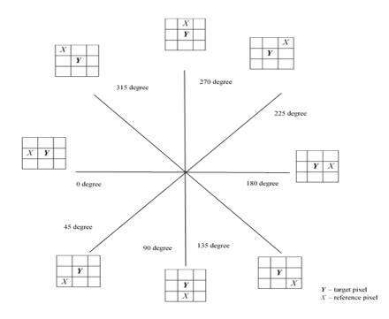
Figure 1. Oriented mask filters for 3x3 neighbourhood of target pixel, Y
