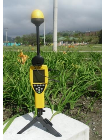
Figure 3. Measuring equipment NARDA NBM-550, with the probe 100KHz-3GHZ and on the front GPS GARMIN
