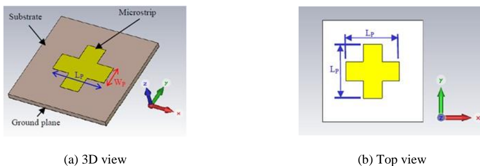
Figure 5. Cross microstrip unit cell
