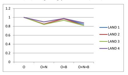
b. Examples of the normalized validation results for the proposed algorithm for blind image quality assessment of landscape images. The algorithm has been tested for original image (O), original image plus noise (O+N), original image plus blur (O+B), and original image plus noise and blur (O+N+B).
