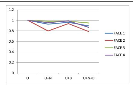
a. Examples of the normalized validation results for the proposed algorithm for blind image quality assessment of face images. The algorithm has been tested for original image (O), original image plus noise (O+N), original image plus blur (O+B), and original image plus noise and blur (O+N+B).
