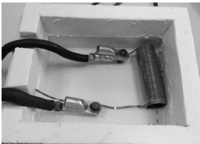
Figure 1. HTS coil connected to the power source in the polystyrene bath for liquid nitrogen filling
