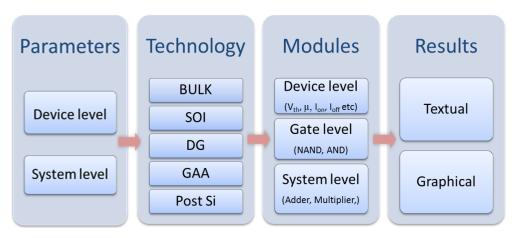
Figure 1. TAMTAMS analysis flow. Three kind of analysis are possible: device level, gate level and system level. Device and system level parameters are used according to the kind of investigation selected by the user. Computed results are reported in a textual or graphical form.
