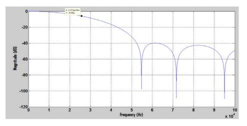
Figure 6. Kaiser filter reponse for sampling frequency of 112 kHz
