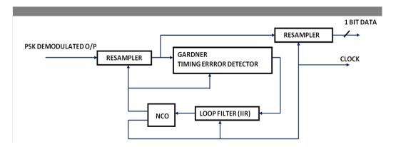
Figure 9. Bit synchronizer block diagram
