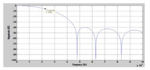
Figure 7. Kaiser filter reponse for sampling frequency of 98 kHz
