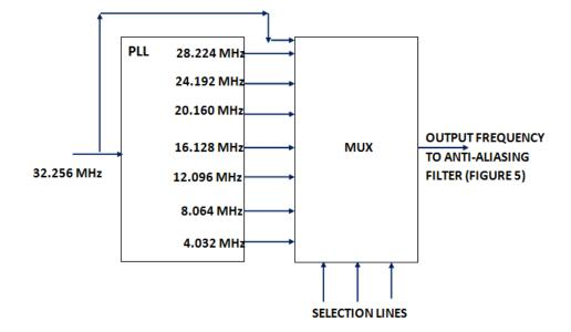
Figure 4. Clock generation on FPGA
