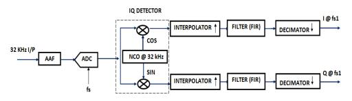
Figure 5. Demodulator front end
