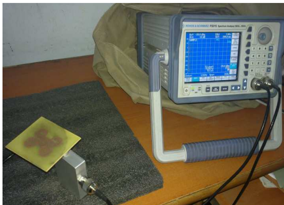
Figure 14 (b). Experimental Testing of RMPA loaded with “SPLIT RING” shaped metamaterial structure on Spectrum Analyzer
