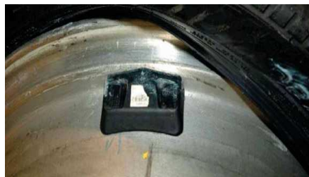
Figure 1 (b). Placement of sensor and transmitter part on the rim of the tyre
