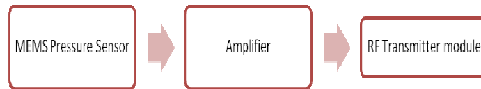
Figure 2. Block diagram of the transmitter block
