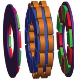
Figure 2. Double-rotor single-slotted stator structure (AFPMSG)
