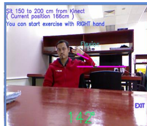
Figure 13. Example of elbow flexion exercise in real-time
