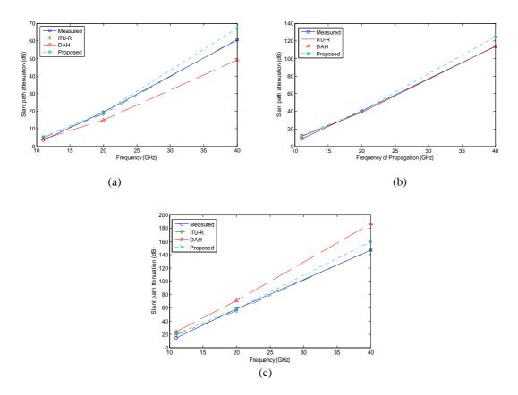
Fig. 9 Relationship between slant path attenuation and frequency for Lagos at (a) 0.1% (b) 0.01% and (c) 0.001% of time.
