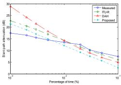
Fig. 6 Comparison of the Slant path attenuation excedanceat12 GHz for Lagos, Nigeria.
