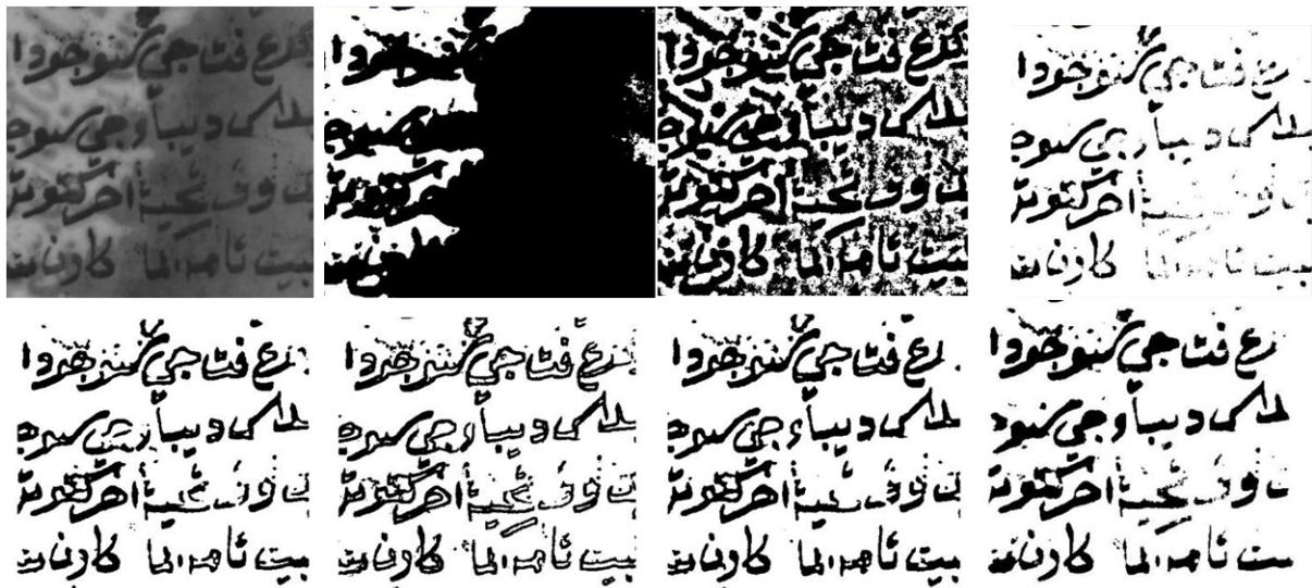
Figure 6. Examples of binarized Jawi ancient document (top: from left to right (original image, otsu, niblack, and sauvola techniques), bottom: from left to right (lu, su, nina, and proposed techniques))
